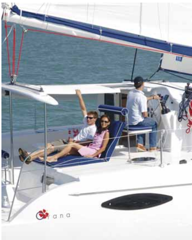
Helm seat and sunlounge are on raised moulding which provides headroom for owner's bunk below.
