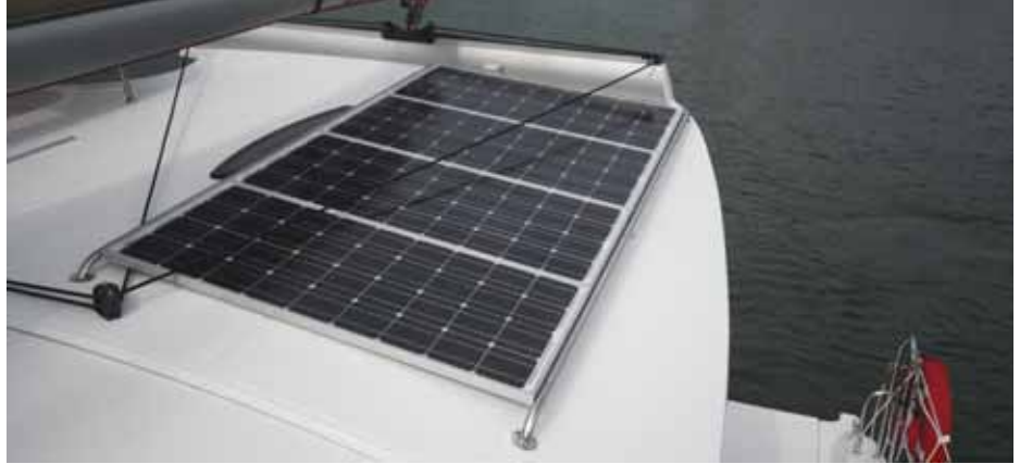
Plenty of power, courtesy of the engine alternators and these four 85-Amp solar panels.
